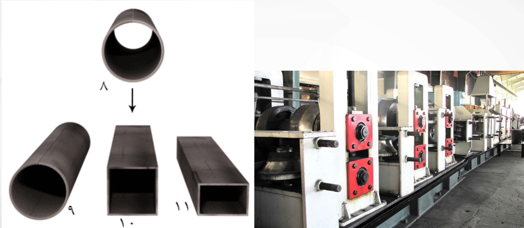
Machine for production of pipes and profiles of heavy steel sections
