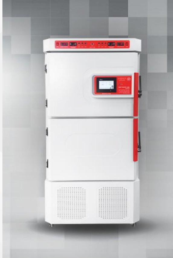
Deep Freezer -80°C with Two Refrigeration Cycles
